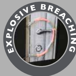
Cutting charge on head locks
