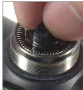
J-5. Apply gentle force on the plastic tab and dial the knob.
