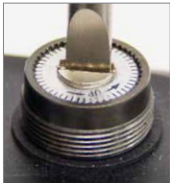
J-3. Use a flat head screwdriver to adjust the windage and elevation.
