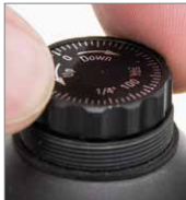
J-4. Apply gentle force on the rim and dial the knob.
